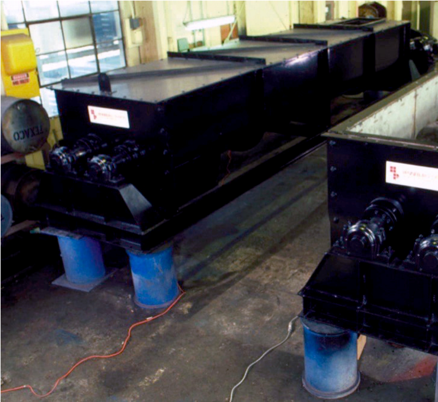
Pugmill mixers in production at Heyl Patterson
