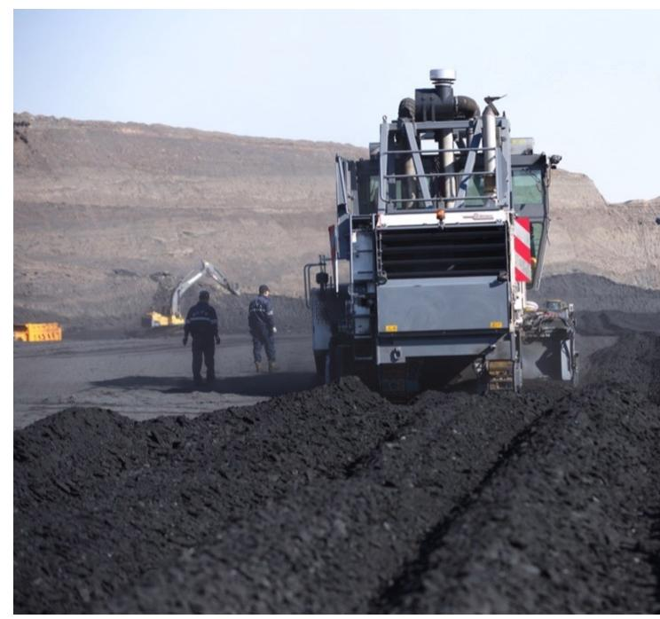
The 2200 SM 3.8 surface miner operates according to the windrowing method: after cutting the material, it deposits it in three windrows behind it.
