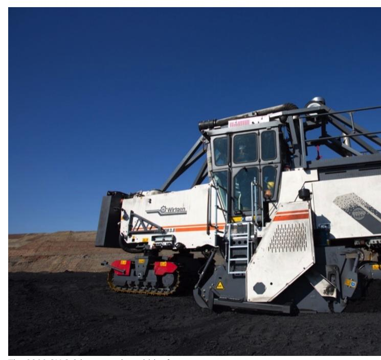
The 2200 SM 3.8 has a cutting width of 3.8 m and a cutting depth of up to 350 mm
