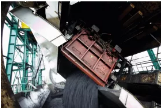
Automated discharge of flat bottom railcar by wagon tippler.
