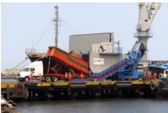
Exporting copper concentrate from Peru direct from truck to ship.
