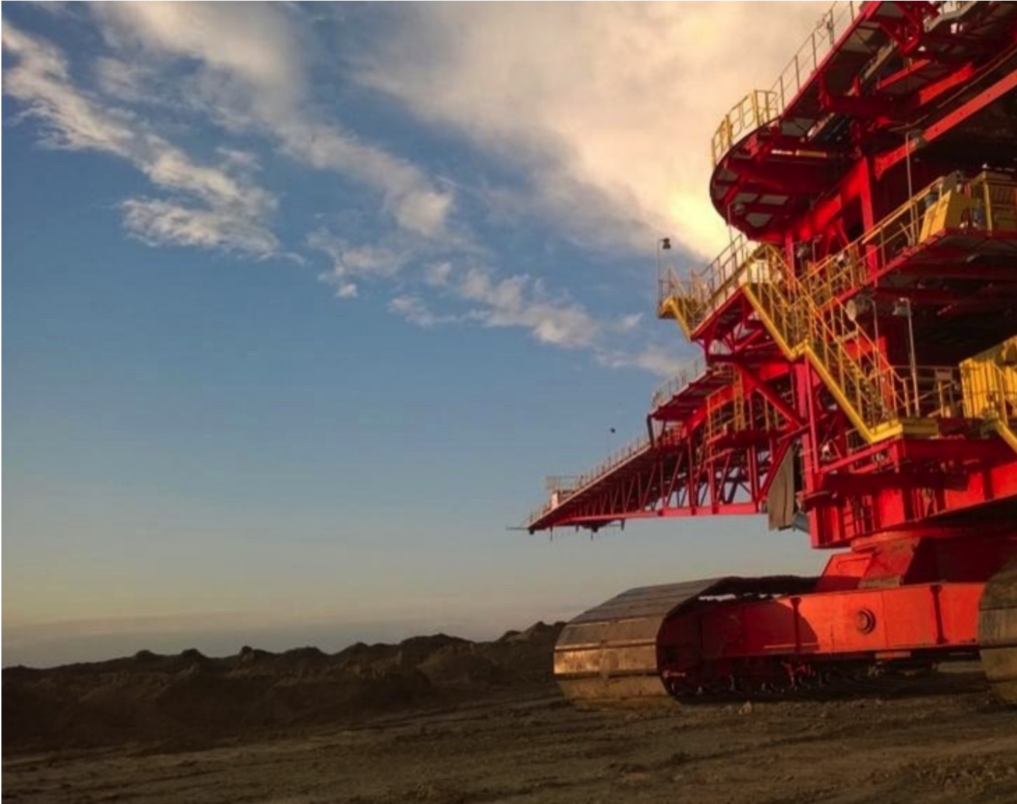
7900 m 3 /h Tenova Takraf spreader at Zhahanaoer open pit mine in China.
