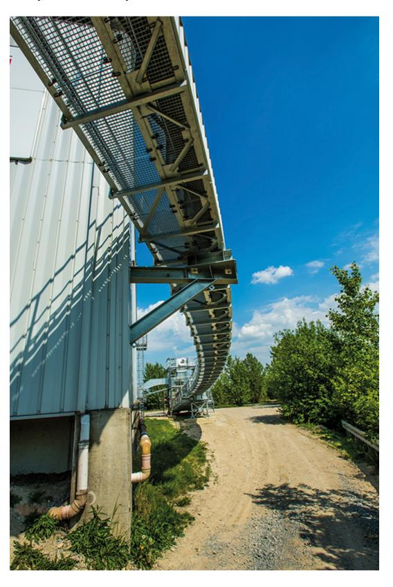
The first support of the pipe conveyor is mounted directly to the storehouse.
