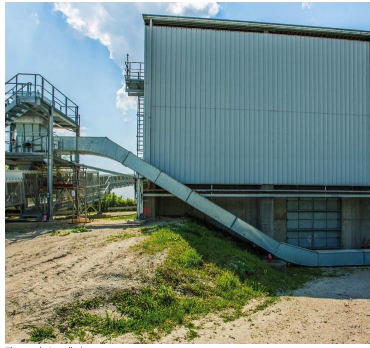
The newly installed system uses a chain belt conveyor to lift the material to the height of the pipe conveyor's loading point.
