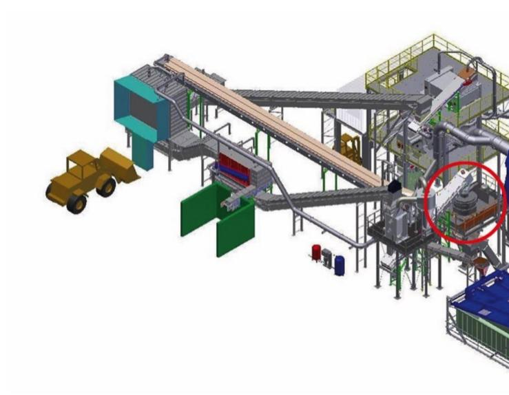
Layout of the fine grain recycling plant. The rotor impact mill is the centerpiece of the entire installation. (Pictures: © BHS)
