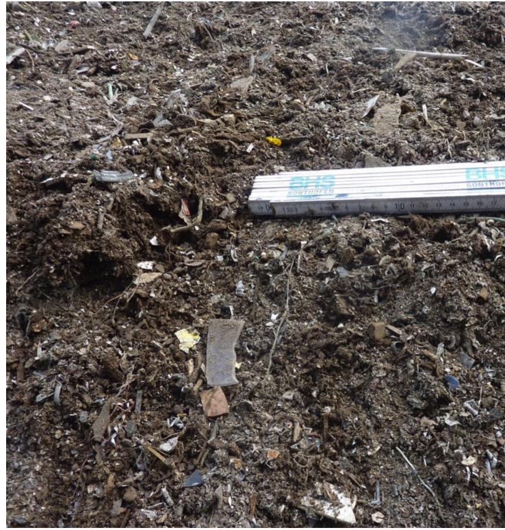
The input material consists of the fine components from coarse shredding.
