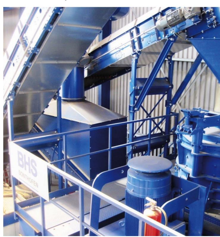
The rotor impact mill of type RPMV in a plant for the fine crushing of shredder waste materials.
