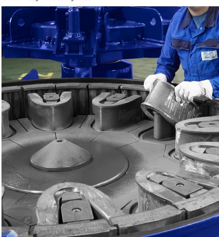
The hammers and the elements of the outer wall are exchanged without tools.
