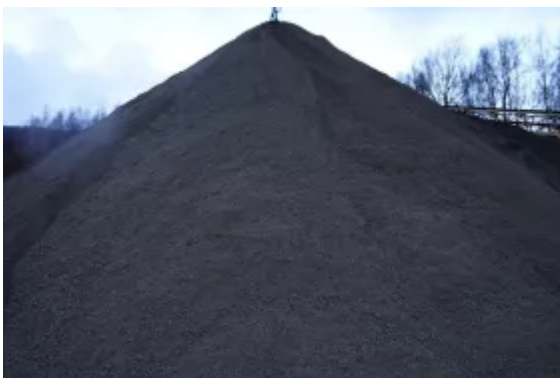
Fig. 1: Early attempts to use this co-generated material as fine aggregate were mainly unsuccessful. However, today the important differences between natural sand and surplus quarry fines are well known and there are examples of the producer successfully overcoming the challenges. (Picture: © Rolands Cepuritis)
