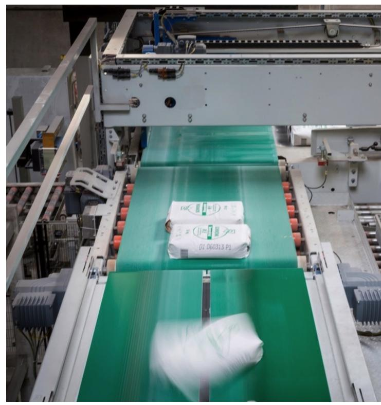
The twin-belt turning device: Two parallel belt conveyors, driven with different speeds during the turning process, bring the bags gently into the required position.
