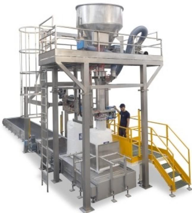
The new net weighing and filling station for single loop bulk bags can fill up to 180/BB per hour. (Picture: ©Concetti)
