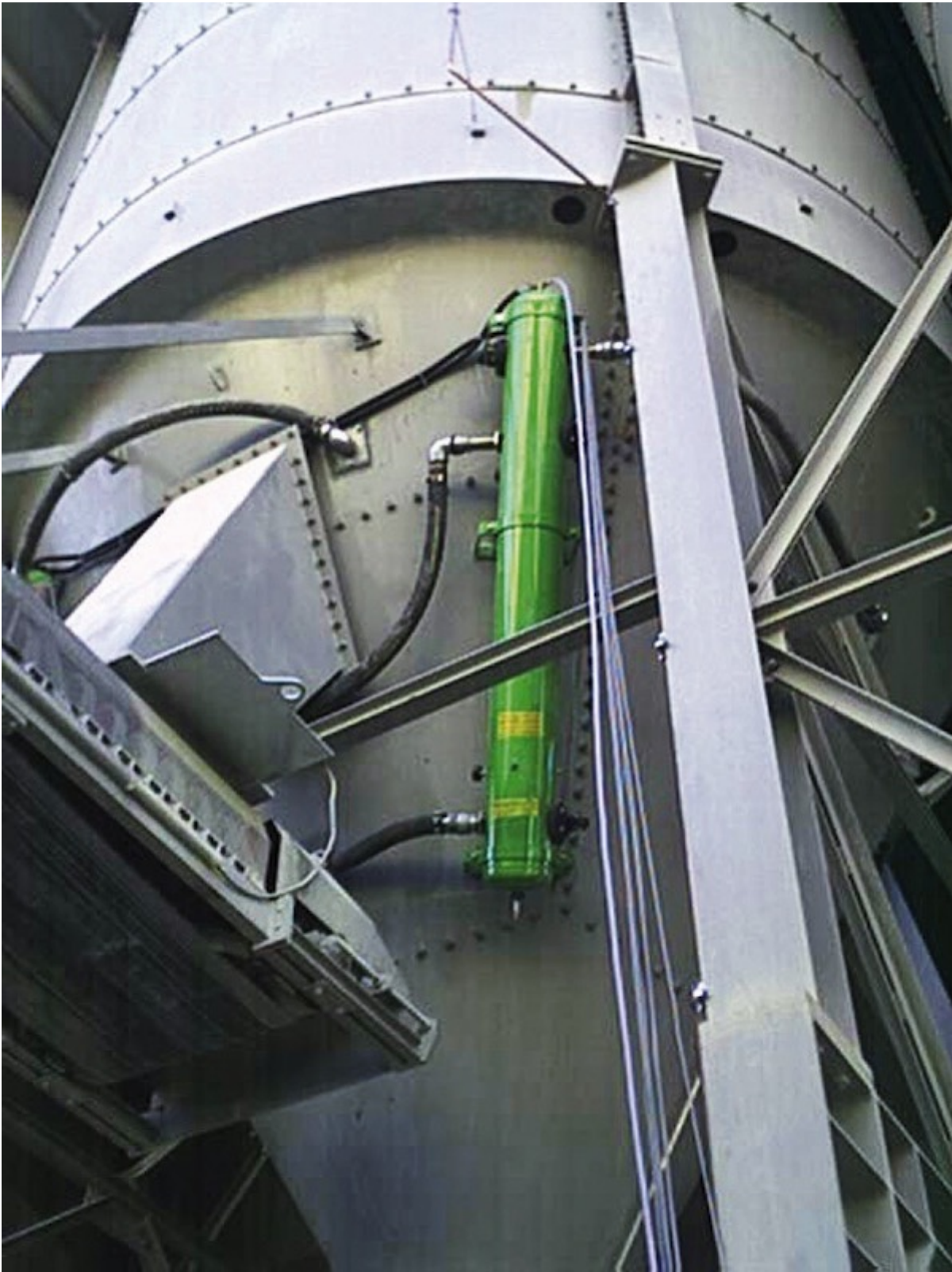
Figl 2: The Matak air cannon system by B+W innovative produkte offers the possibility to install lance nozzels at critical zones. (Picture: © B+W Innovative Produkte)
