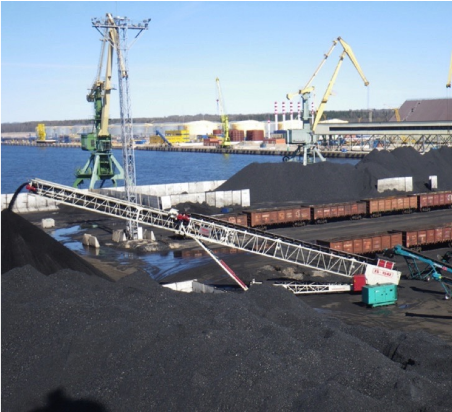
Fig. 1: Mobile system can be a cost efficient alternative to stacker/reclaimer systems and offer a great mobility and flexibility. (Pictures: © Telestack Ltd.)
