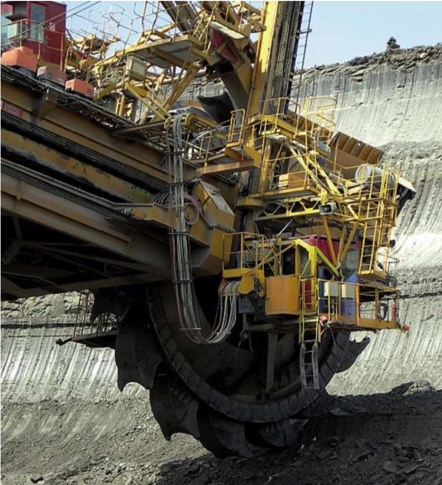
Fig. 1: Rolling bearings in bulk material conveying applications are most confronted with high specific loads in combination with low rotational speeds and subjected to liquid and solid contamination. (Picture: Shutterstock)
