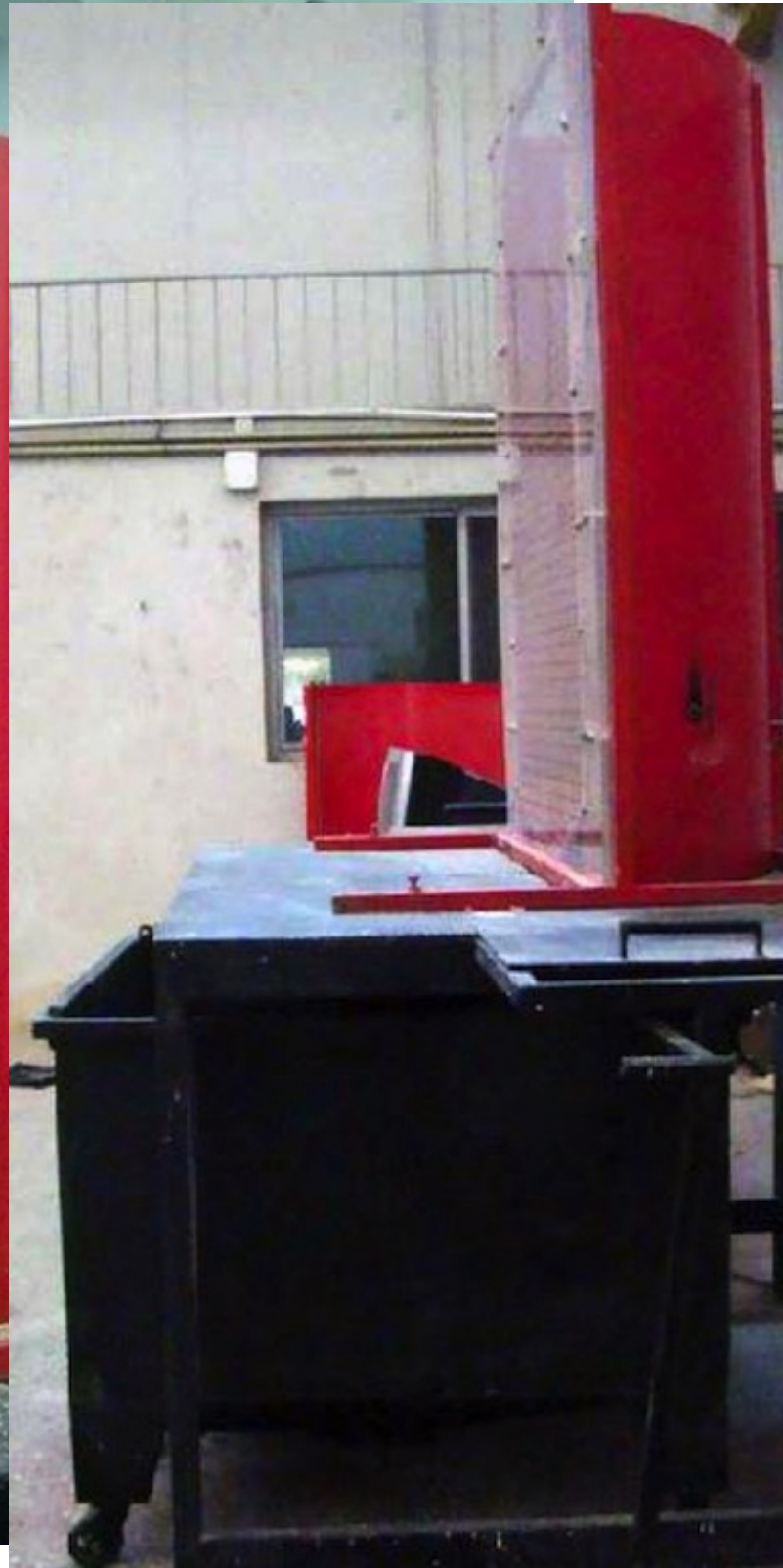
Fig. 3. View of the model silo showing plexiglas front.
