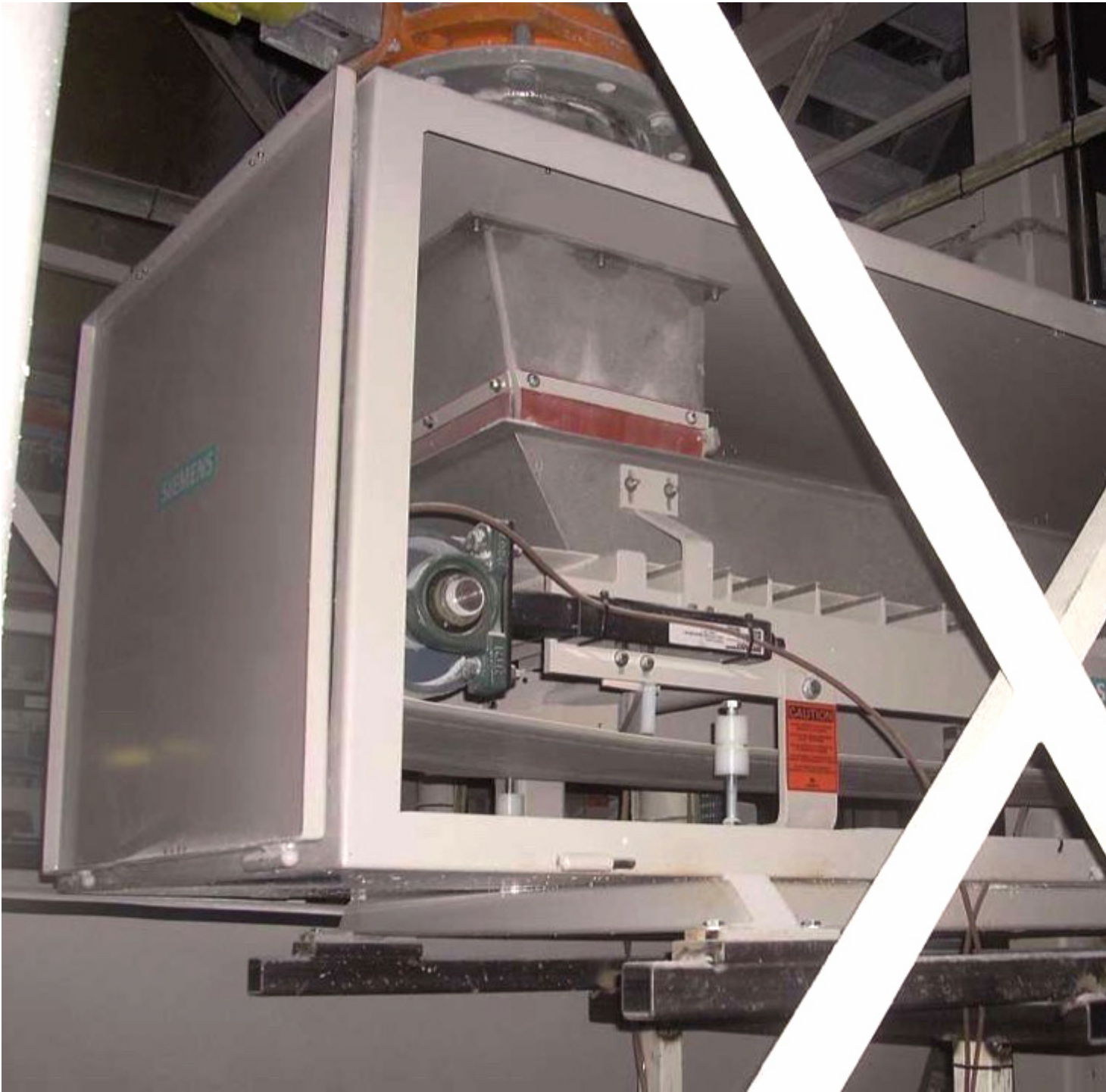
Fig. 1: After a simple installation of the weighfeeder, maintenance requirements were significantly reduced. (Pictures: Siemens AG)
