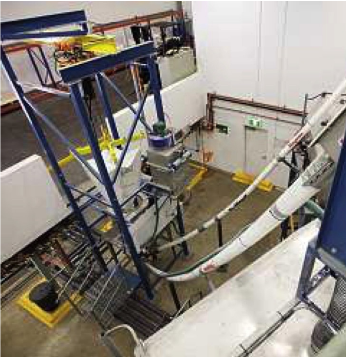
Fig. 3: Powder remains enclosed from the time it is received until it enters the mixing tanks.
