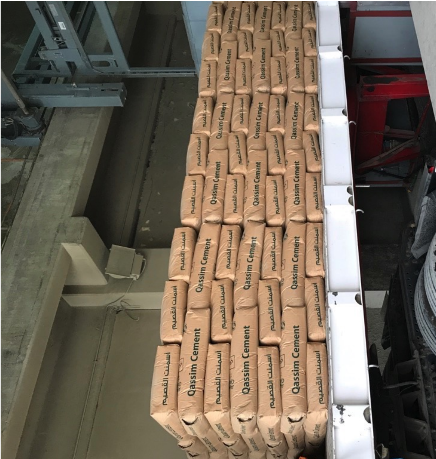
Fig. 5: The hard physical work of manual loading is omitted thanks to automatic loading and simultaneous palletising.
