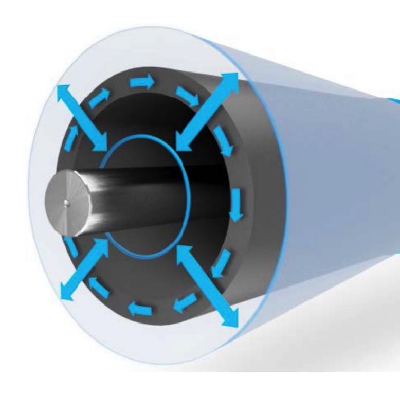
"This is unlike conventional belt trackers that slide over the belt surface causing possible abrasion and belt damage rather than adopting free rotation. Conventional belt trackers, with tapered edges, never idle and are always in a braking mode.
