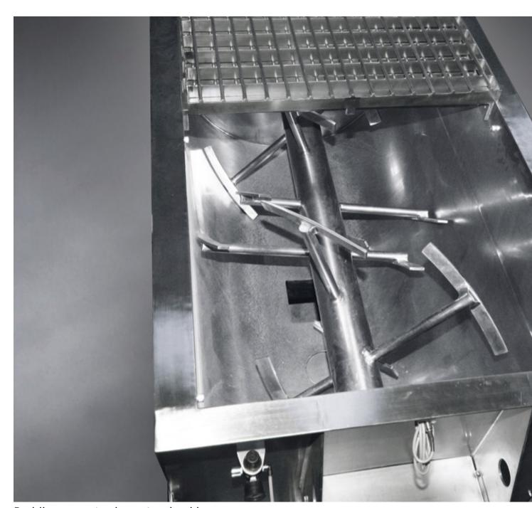
Paddle geometry is customized by application for efficient performance.
