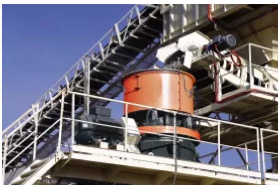
Fig. 3: The Kulai quarry uses a CS series cone crusher for secondary crushing.
