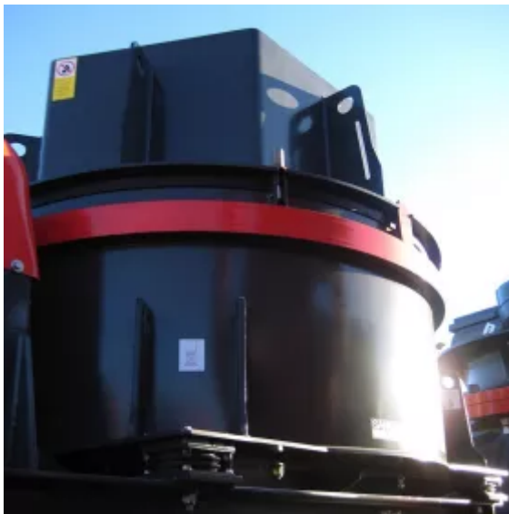
Fig. 6: The CV series VSI shaft impactors have been developed to ensure consistent product shape and size.
