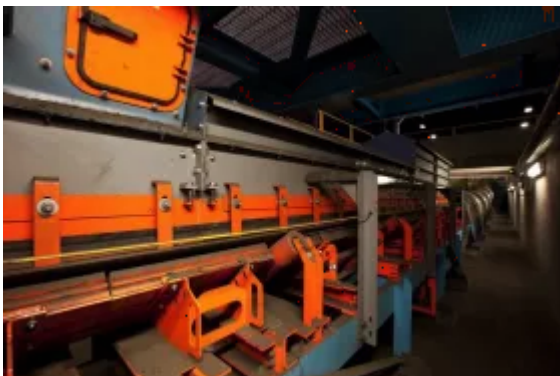
Fig. 3: Martin® ApronSeal™ Skirting is a dual-sealing system, with a primary seal clamped to the steel skirtboard and an “outrigger” strip to capture fines and dust.
