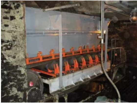
Fig. 3: The EVO External Wear Liner is designed to remove the material burden from the dust containment system.
