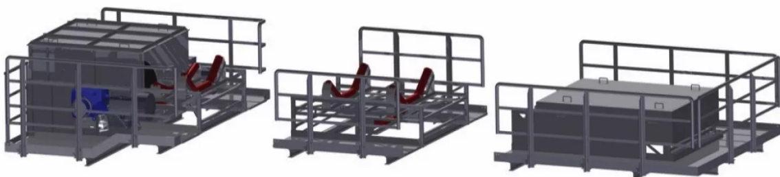
Fig. 2: The modular system developed by H+E Logistik consists of three basic components: the drive, the bridge and the reverse module.
