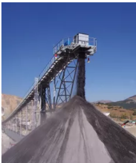
Fig. 1: Modular belt conveyor systems enable fast installation and dismantling and also increase reusability of components for temporary projects. (Picture: H+E Logistik GmbH)
