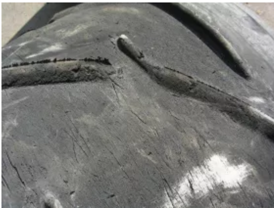
Fig. 2: Chevrons as high as 25mm or 32mm can wear almost completely flat in a remarkably short time.
