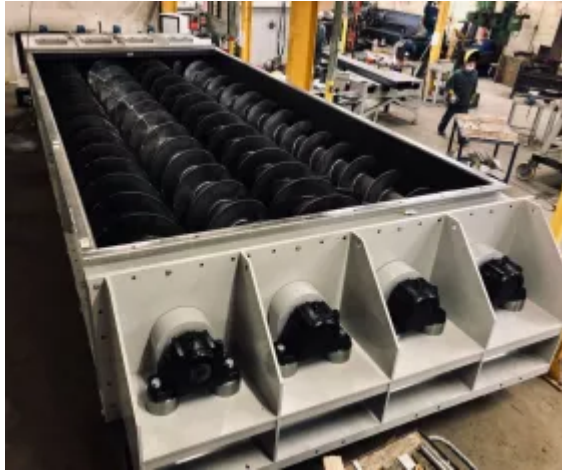
Quadruple Screw Feeder designed to work with poorly flowing refuse to provide a regular feed.
