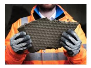
As materials are washed and graded, the water from that process accumulates silt and other residues to form a sludge. A challenging material to process, that sludge is pumped under high pressure into the CDE ProPress, which consists of a sequence of plates, the composition of which forms a series of chambers.
