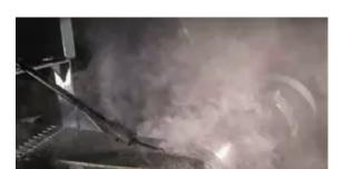
Friction heat between rolling components can be extreme enough to light both the material and belt.
