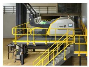
UniSort Finealyse®+ for sorting fine-grain bulk material like plastic mixes, copper scrap and heavy metal and non-ferrous metal concentrates.
