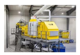
The new STEINERT PLASMAX® | LIBS enables recycling firms to take aluminium recycling to the next level and to specifically produce high-grade alloy classes ready for the furnace. (Pictures: ©STEINERT)
