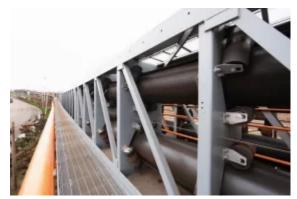
BEUMER Group is supplying a 4,150 t/h bi-directional pipe conveyor to the Port of Saguenay. The system will be installed inside an enclosed gallery structure for ease of maintenance during the winter months. (Picture: ©BEUMER Group GmbH & Co. KG)
