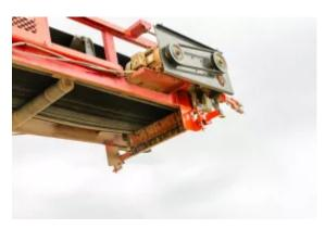
The Martin® SQC2S<sup>™</sup> Secondary Cleaner removes dust and fines in scratches and divots not cleared by the primary cleaner.
