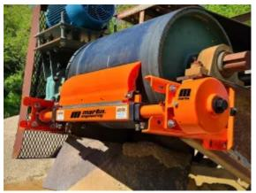
The Martin  $\$  QC1+ $^{\text{m}}$  Cleaner HD can use a twist tensioner for consistent pressure through the blade life.
