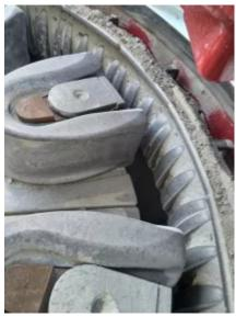
The alternating direction of rotation of the Rotor Impact Mill ensures uniform wear across all components, reducing system maintenance requirements.
