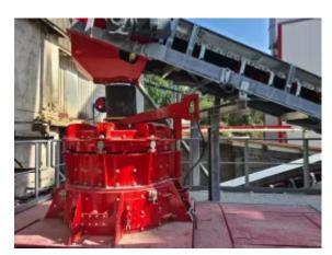
Since 2019, Dachser has been using BHS rotor impact mill type RPM 1513 to produce sand from excess gravel. (Pictures: ©BHS-Sonthofen GmbH)
