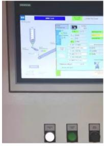
The control system features powerful frequency converters for energyefficient operation of the machines and a modern user interface with touch screens.
