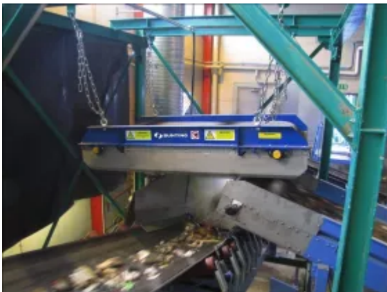
Bunting Permanent Overband Magnet in a recycling operation (Pictures: ©The Bunting Magnetics Co.)
