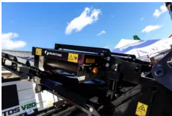
Bunting Permanent Overband Magnet on a mobile crusher
