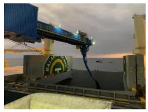
The material slides down a telescopic tube into the cargo hold.
