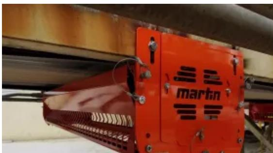
Return roller guards ensure detached rollers don't pose a hazard to workers or harm the system.
