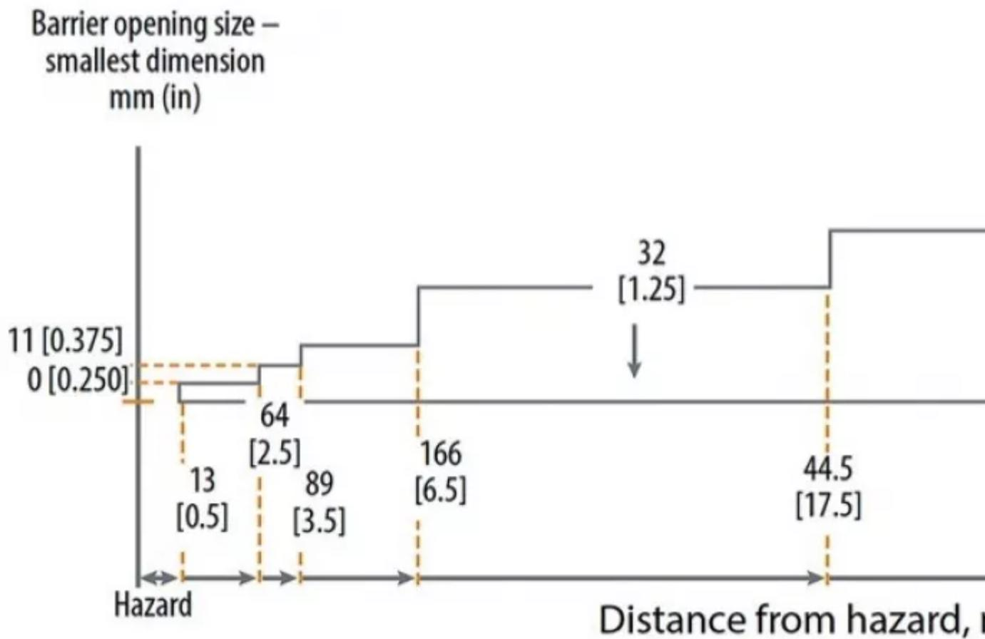
Reach-in hazards (“breaking the plane”) can apply to both the mesh size and the height
