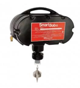
This mechanical instrument uses a weight-and-cable to work like an automatic measuring tape: The sensor lowers a cable with a weight (also called a bob or probe) attached to its end into the vessel. The sensor determines the material's level by measuring how much cable has been let out when the weight reaches the material's surface; then the sensor retracts the cable and returns the weight to the vessel's top.
