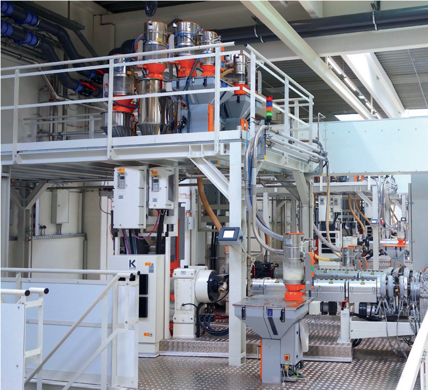
Fig. 4: The 7 layer foil machine is constructed in three functional levels on top of each other. On the lowest level (not visible here) there are three
