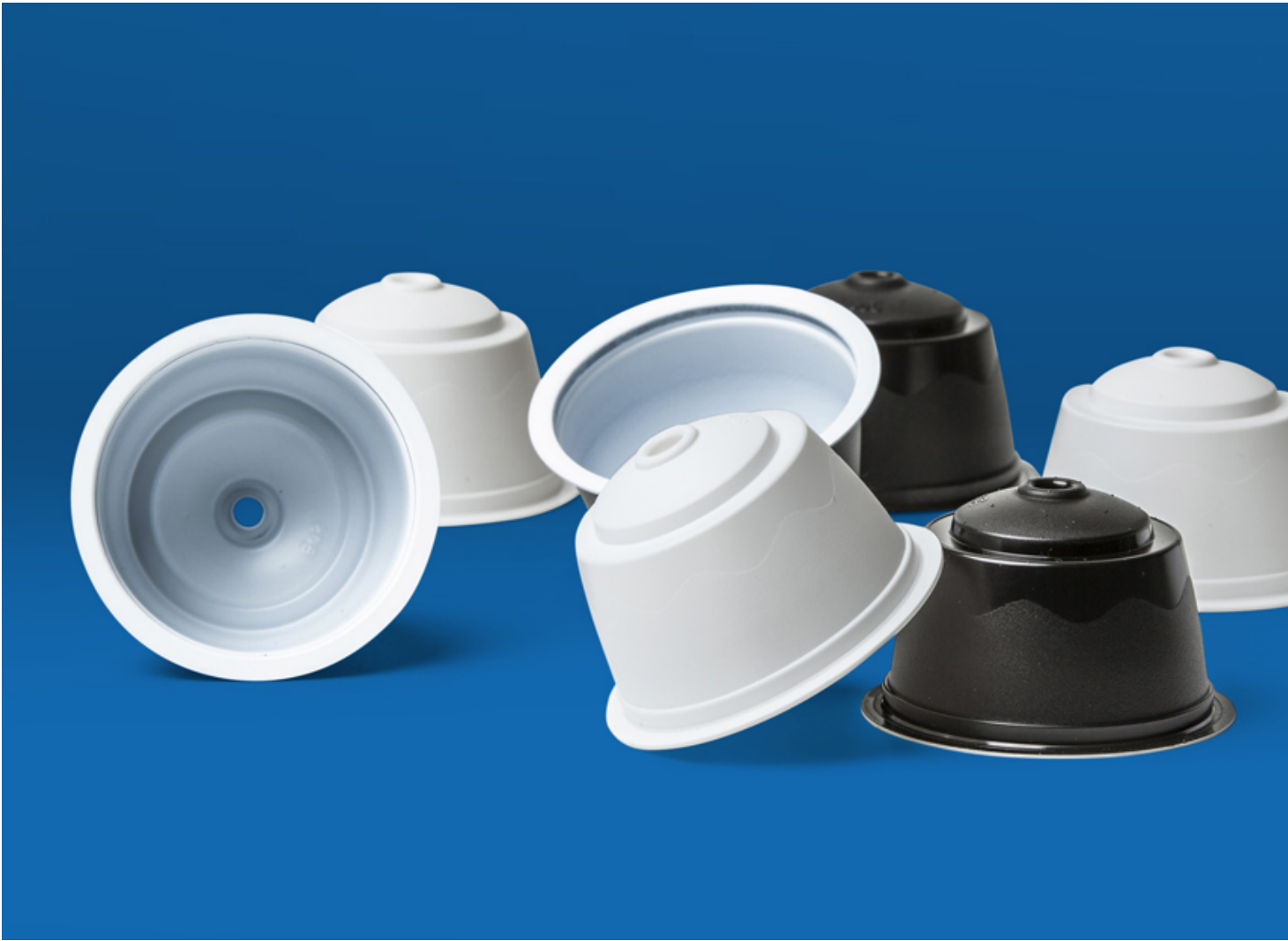
Fig.1: Capsules made of a 7-layer composite foil are the modern way of storing coffee in portions. The film combines barrier properties and recyclability
