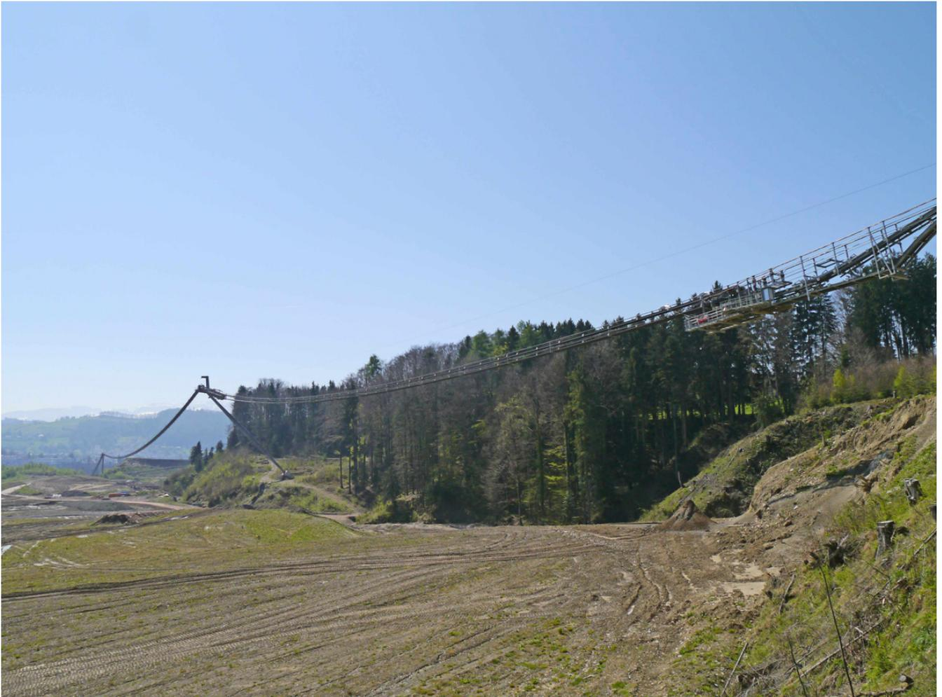
Relocating the discharge point of Tüfentobel RopeCon<sup>®</sup> in various stages was part of the overall project plan from the very beginning. The idea was to discharge the material at all times as close as possible to the location where it was to be used.
