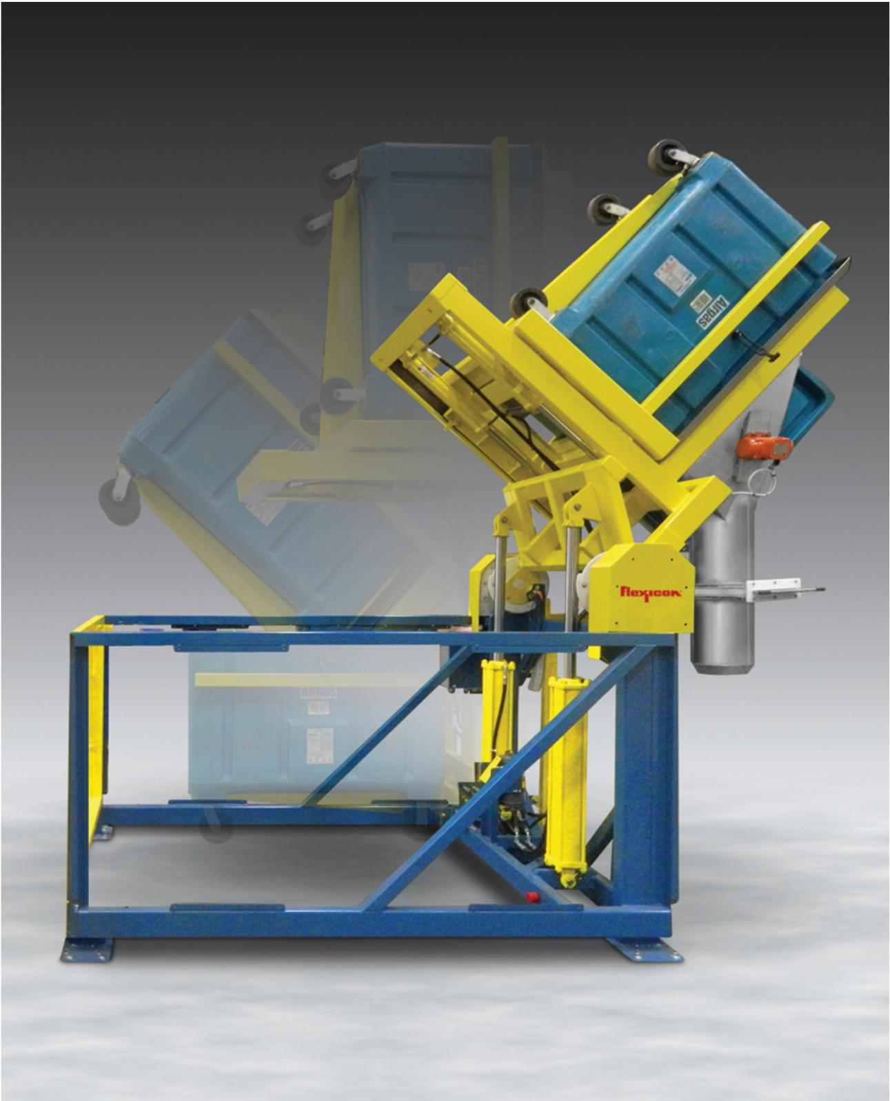
A new TIP-TITE® Tipper for mobile bins transfers bulk material into process equipment and storage vessels dust-free at controlled rates.
