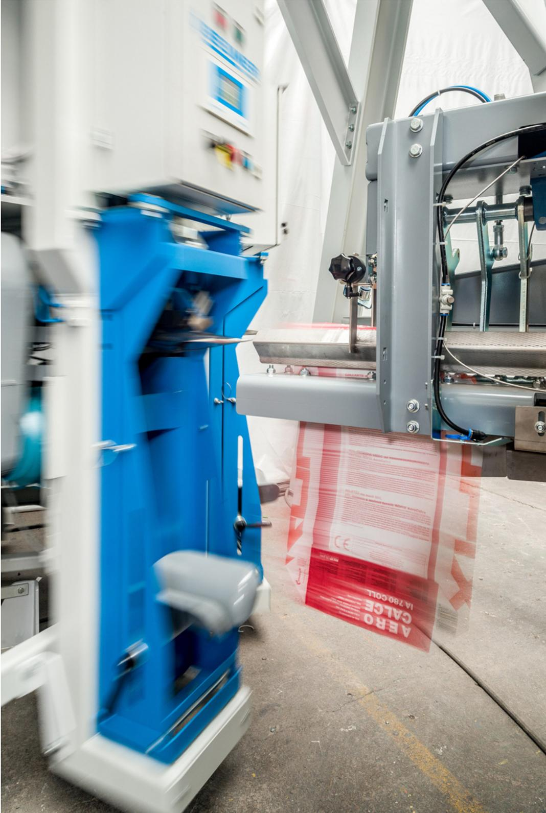
Fig. 3: The gripping arm is supported on both sides. This ensures smooth running even under load.
