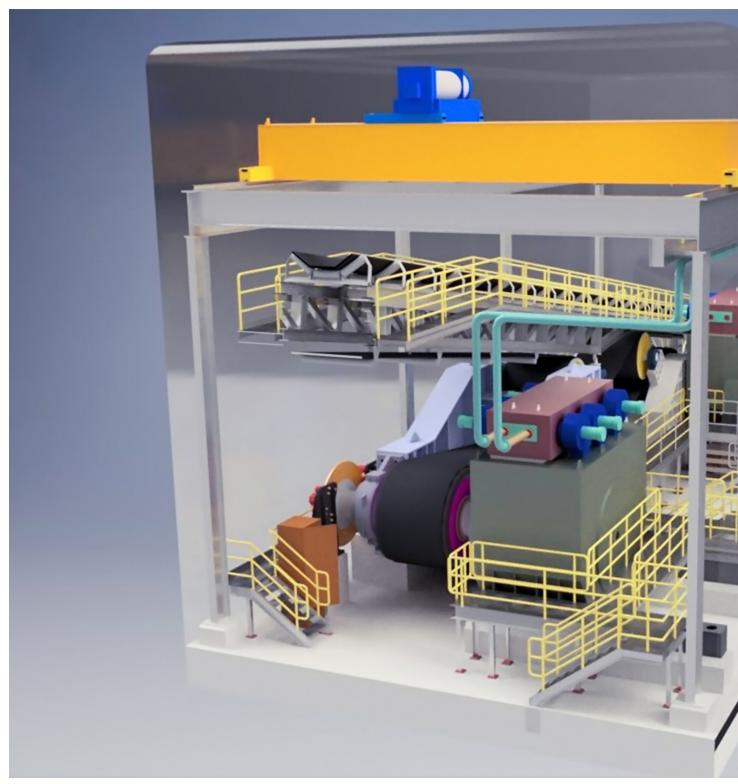
3D rendering of the Oyu Tolgoi underground drive chamber for one of the four slope conveyors with 2 x 5.5 MW gearless drives.
