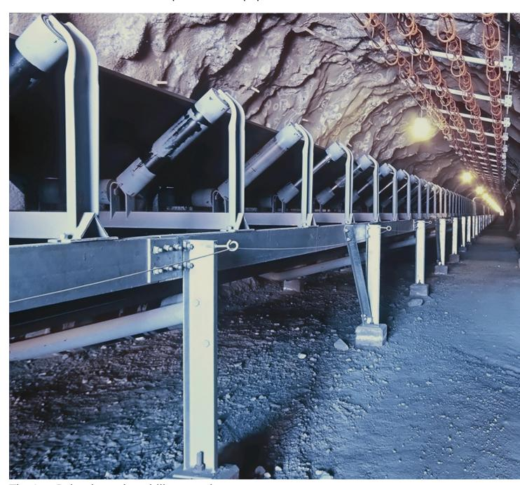
The Los Pelambres downhill conveying system which was developed by thyssenkrupp transports copper ore over a total distance of 12.7 km through a tunnel system.
