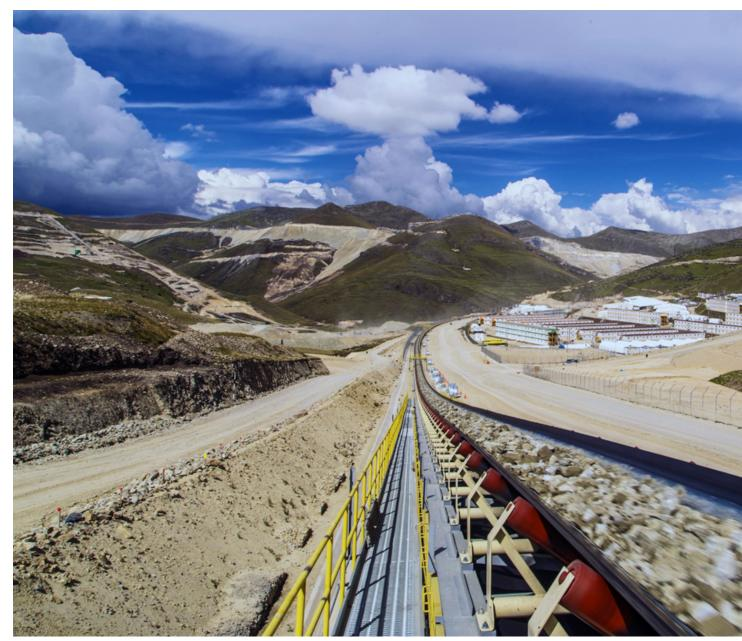
The Las Bambas overland conveyor system in Peru transports 9,400 tons of copper ore per hour over a distance of more than 5.5 km.
