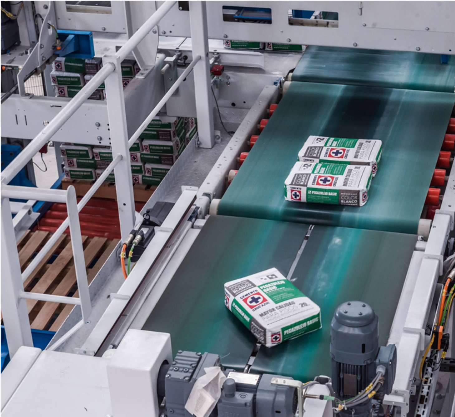
Picture 7: The twin-belt turning device accurately positions the bags quickly and gently.
