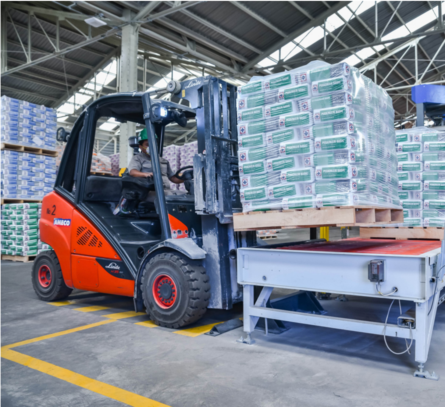
Picture 10: Picking up the palletised and packaged products with a fork-lift truck and delivering them to the outgoing goods.
