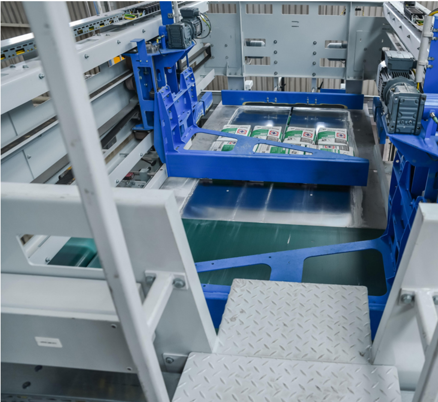
Picture 8: The BEUMER palletpac layer palletiser can stack the bags in a 8- or 10-bag pattern onto pallets of 1,220 x
