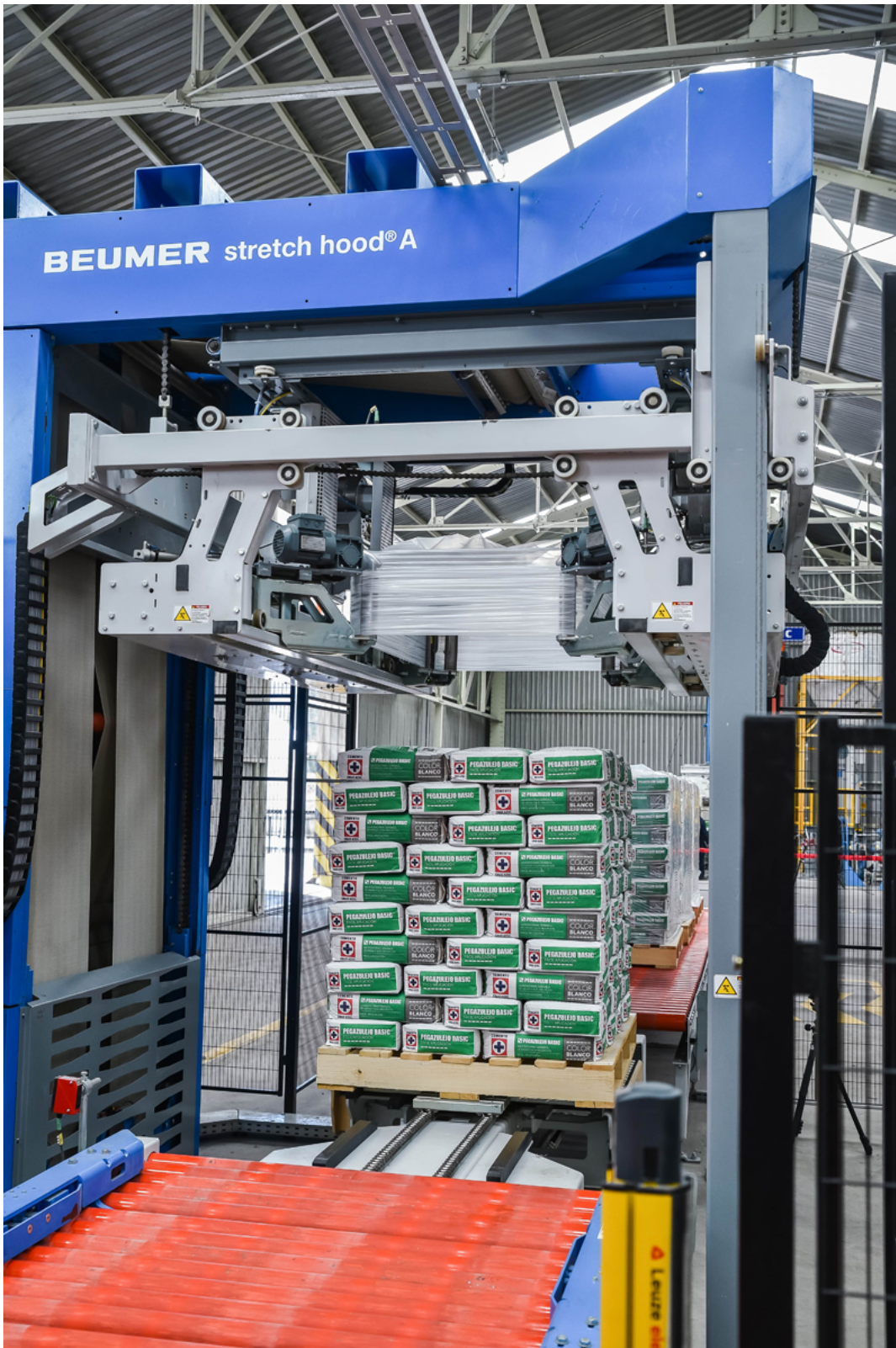
Picture 9: The BEUMER stretch hood A packages the bag stacks with a stretch film hood. This protects the product against damage during transportation and atmospheric influences.
