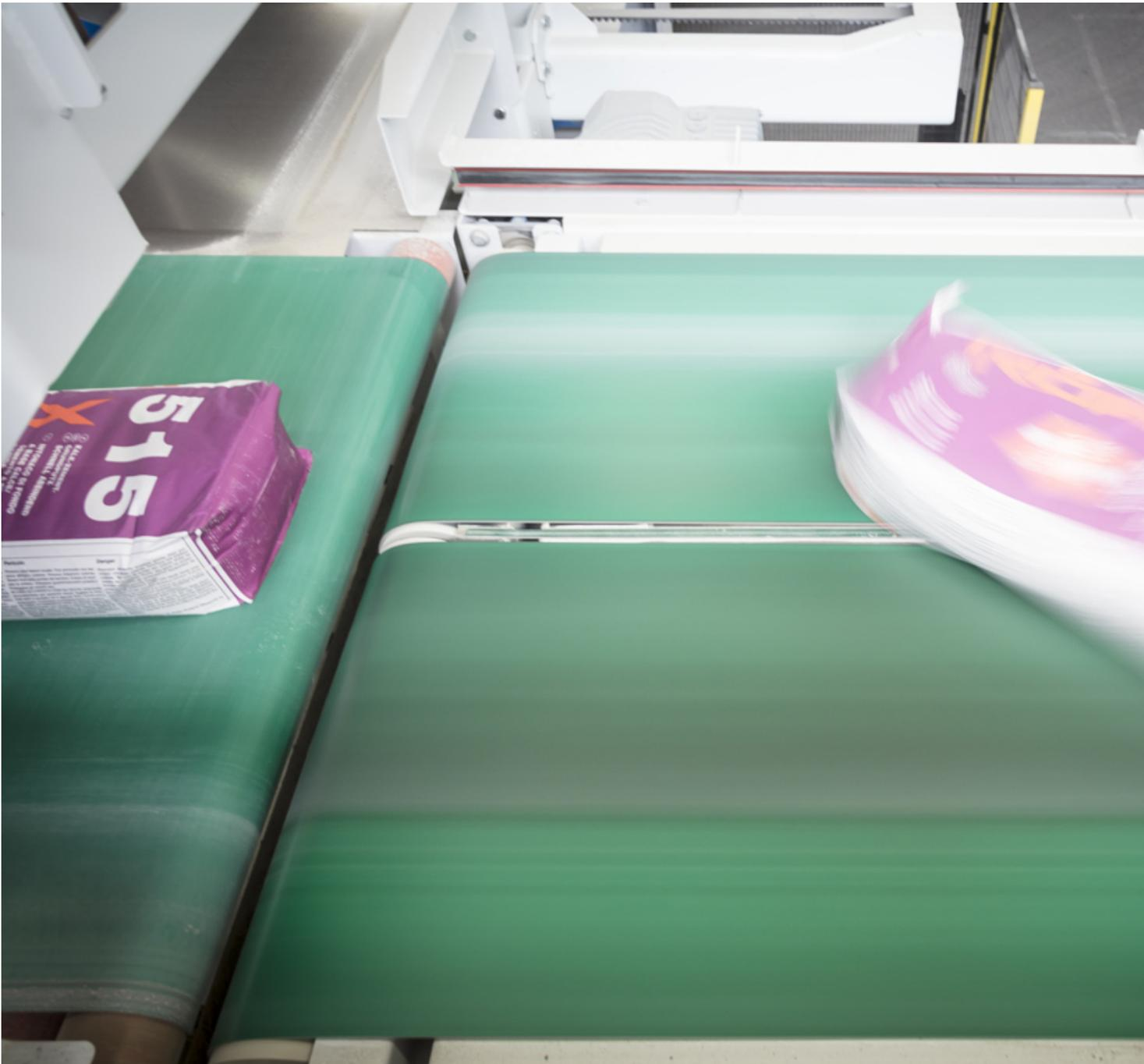
**Picture 5:** The bags are turned fast and gently in the required position by the twin-belt turning device and then palletised.
