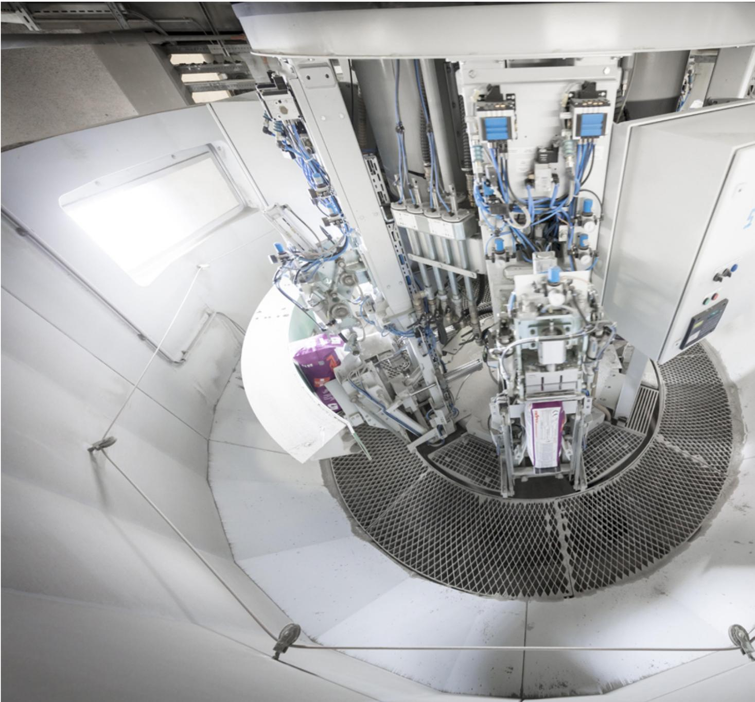
**Picture 2:** BEUMER Group supplied the entire line from one single source. This includes the BEUMER fillpac R that fills material efficiently into the bags. A calibrated electronic weighing unit ensures exact degrees of filling.
