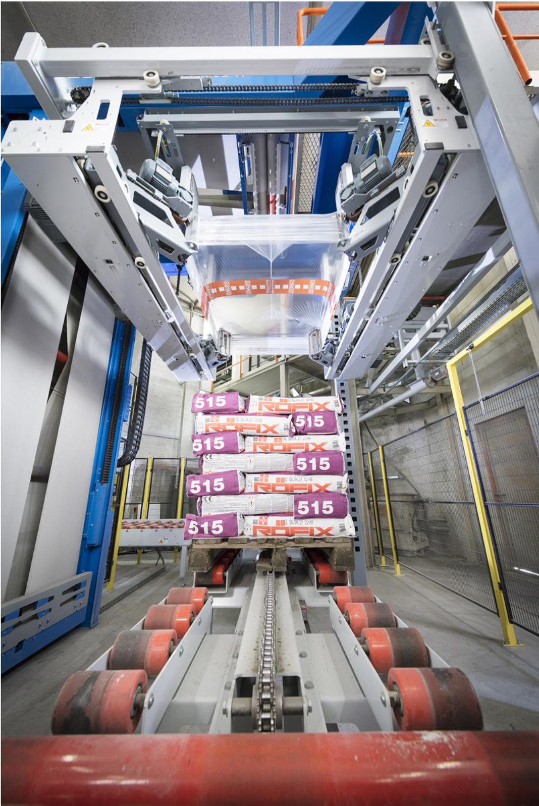
**Picture 7:** The BEUMER stretch hood A places a stretch hood over the palletised products. This increases load stability. And it displays the products efficiently which means optimal brand presentation.
