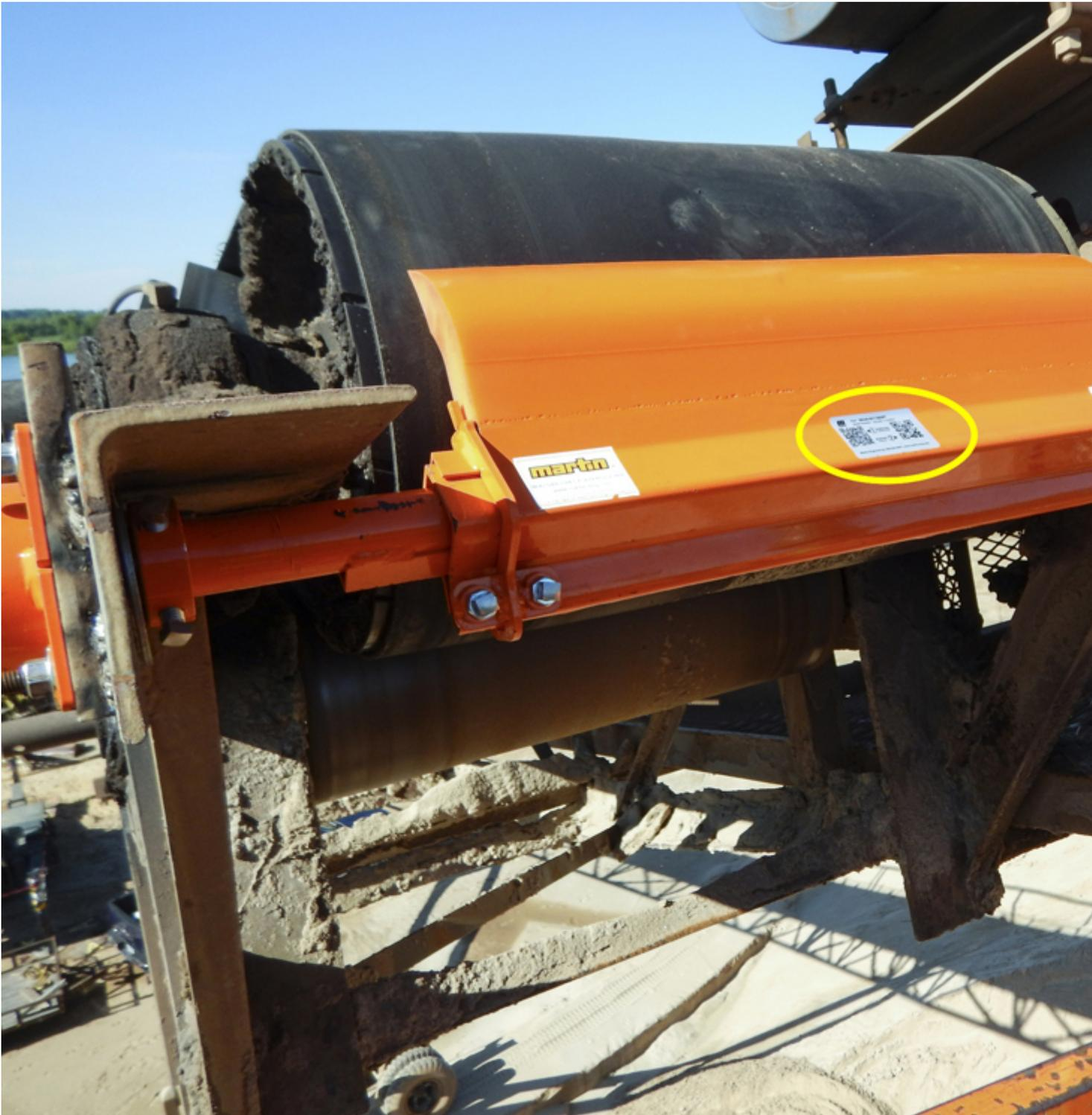
Martin Engineering has introduced data tracking and analysis codes on conveyor belt cleaners.
