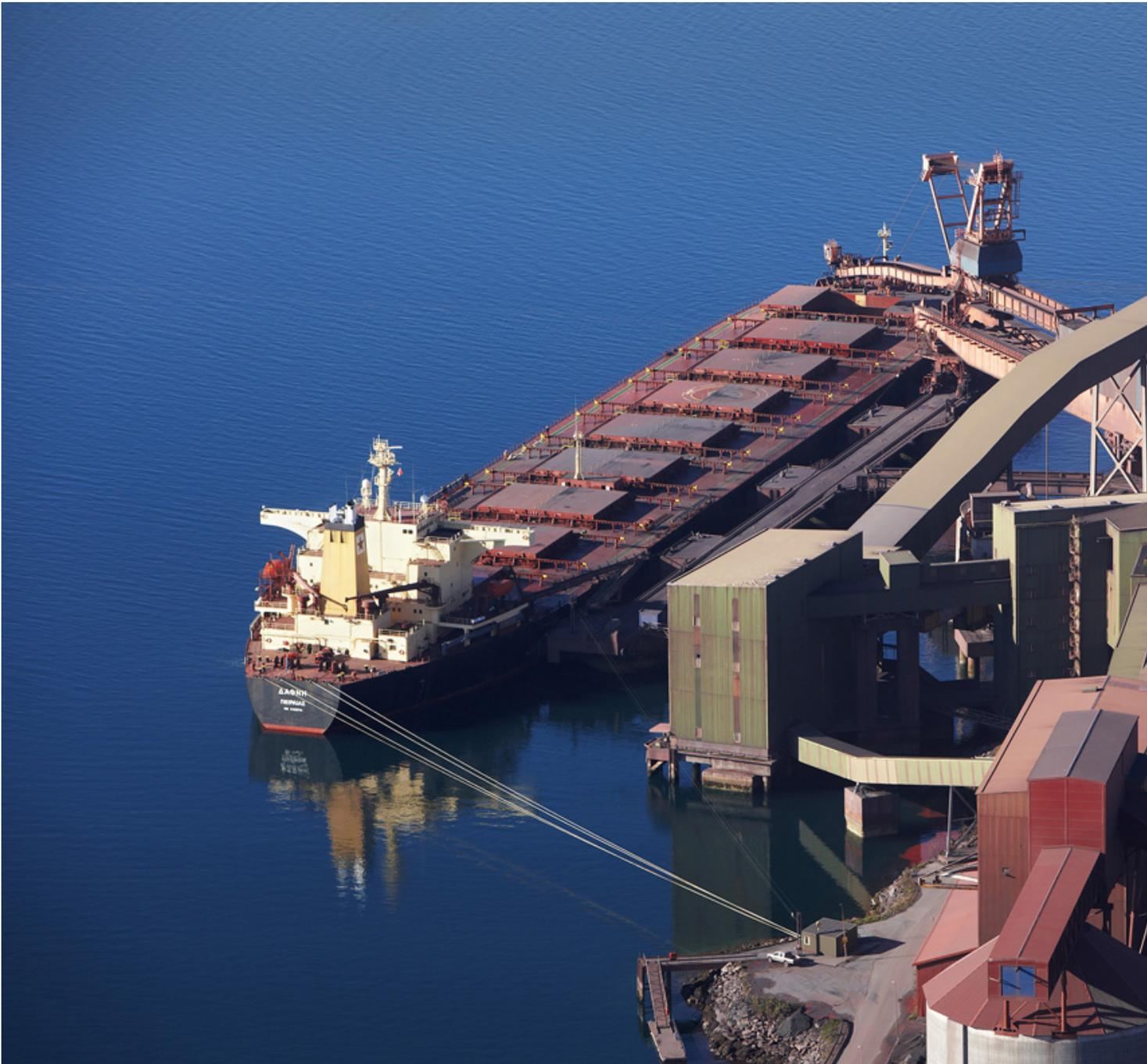
Inside the ship loaders, conveyor belts transport bulk cargo from land to ship.
