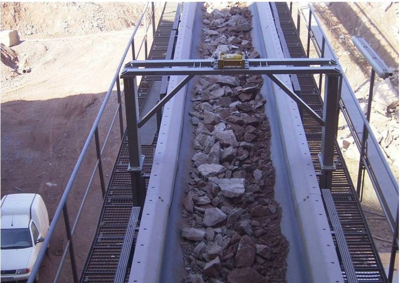
The non-contacting belt scale LB 472 can be installed directly after bunkers,
