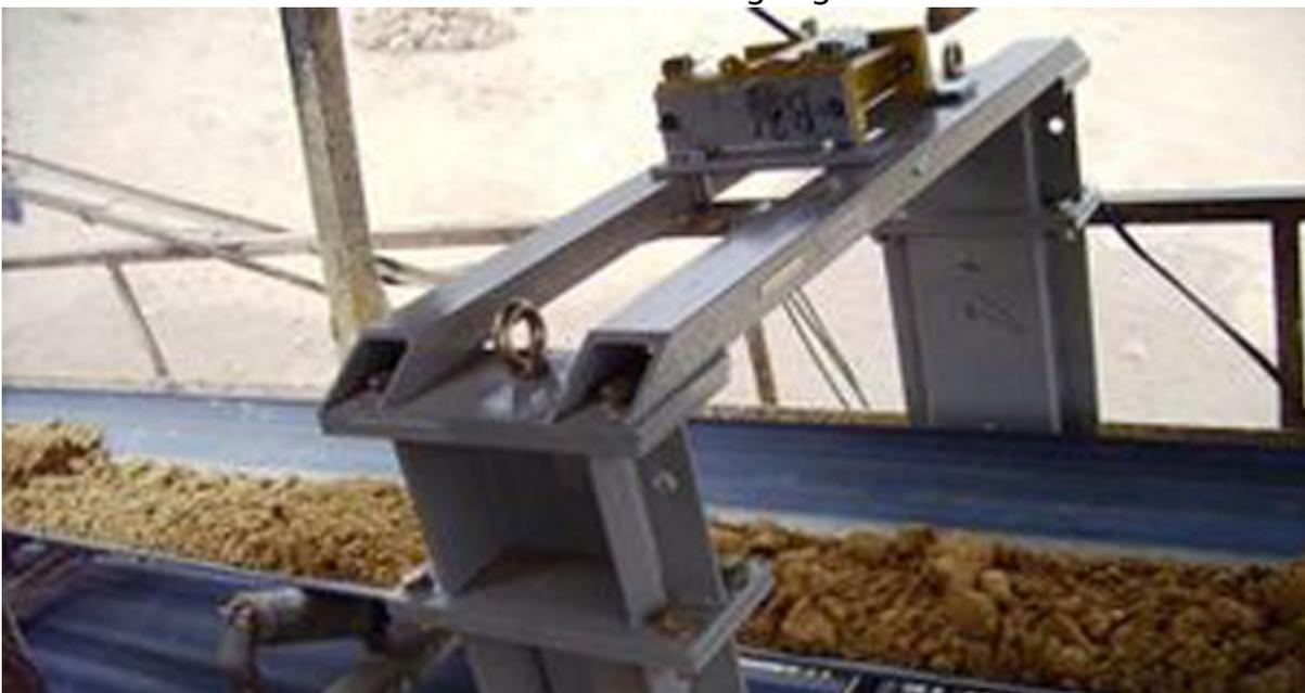
**Customized** On request, we supply the components together with a special mounting frame for installation of the detector and shield. The robust steel frame is optimized in terms of radiation protection and stability and ensures a reliable measurement. By applying the optimal arrangement for different options of sources and detectors we find the best solution for our customers.
