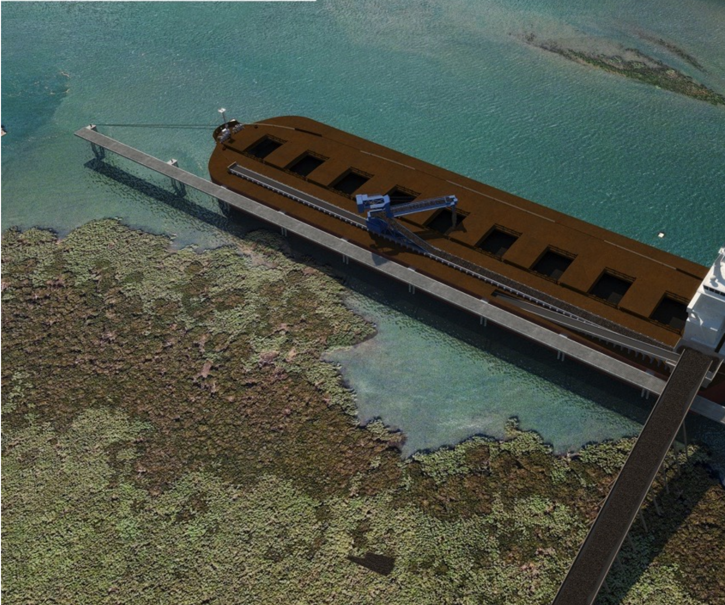
Transmax loading from shore conveyor (graphic representation).
