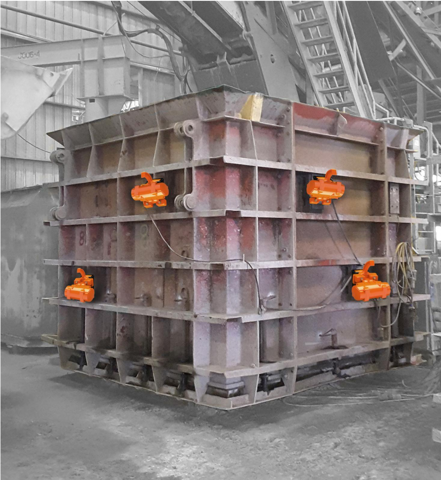
The powerful high-speed vibrator improves material consolidation for exceptional strength and finish.
