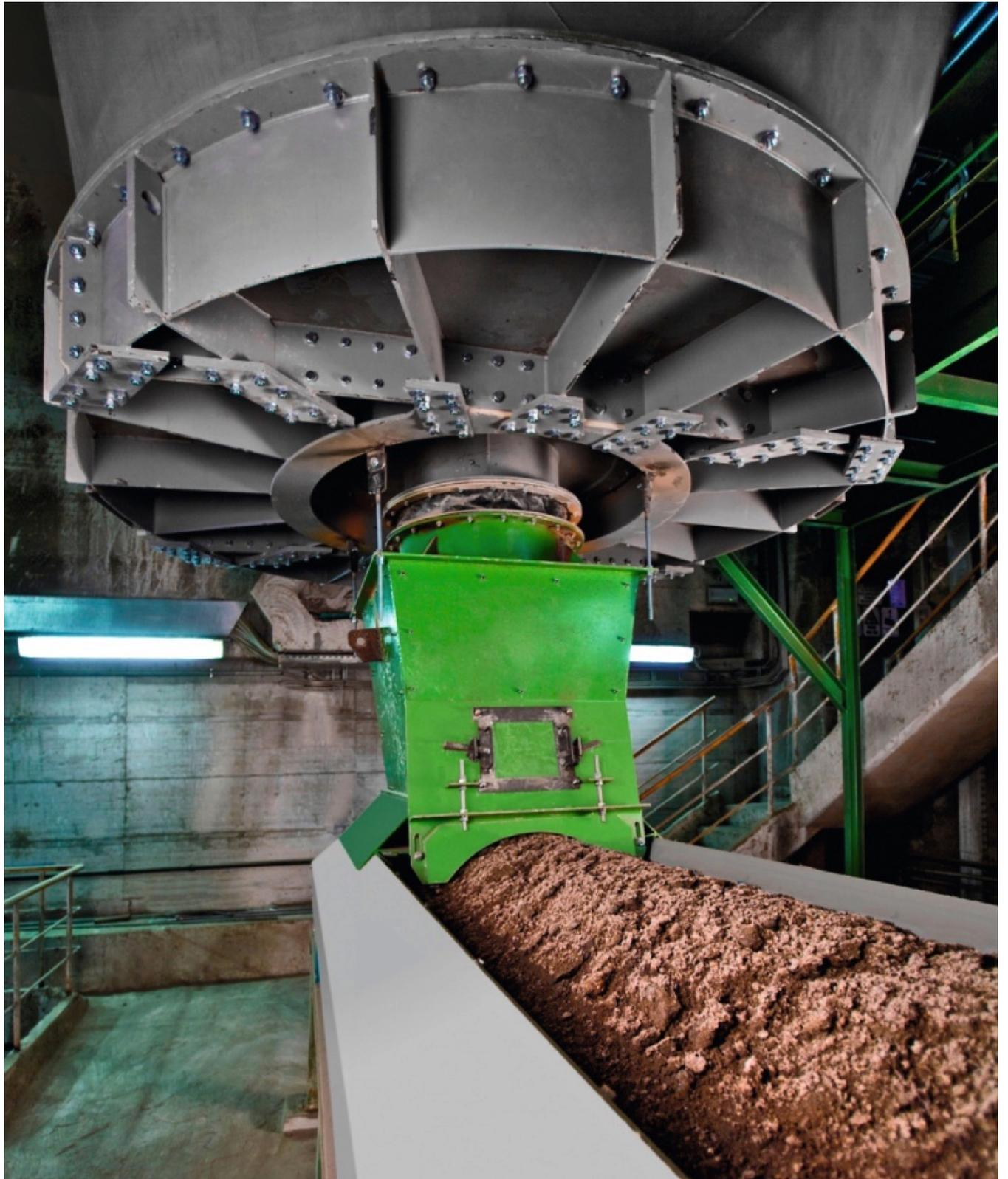
Two CENTREX machines will be extracting a mixture of limestone and clay as well as iron ore from silos.
