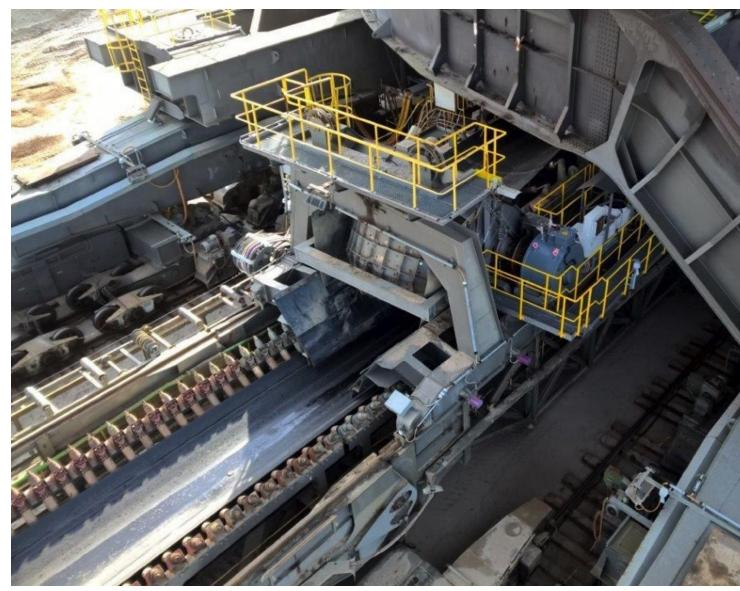
In a pilot project, the new gearless solution was installed on a high capacity (15.000 t/h) discharge conveyor of a bucket chain excavator in parallel with the existing geared drive (Picture: ABB)
