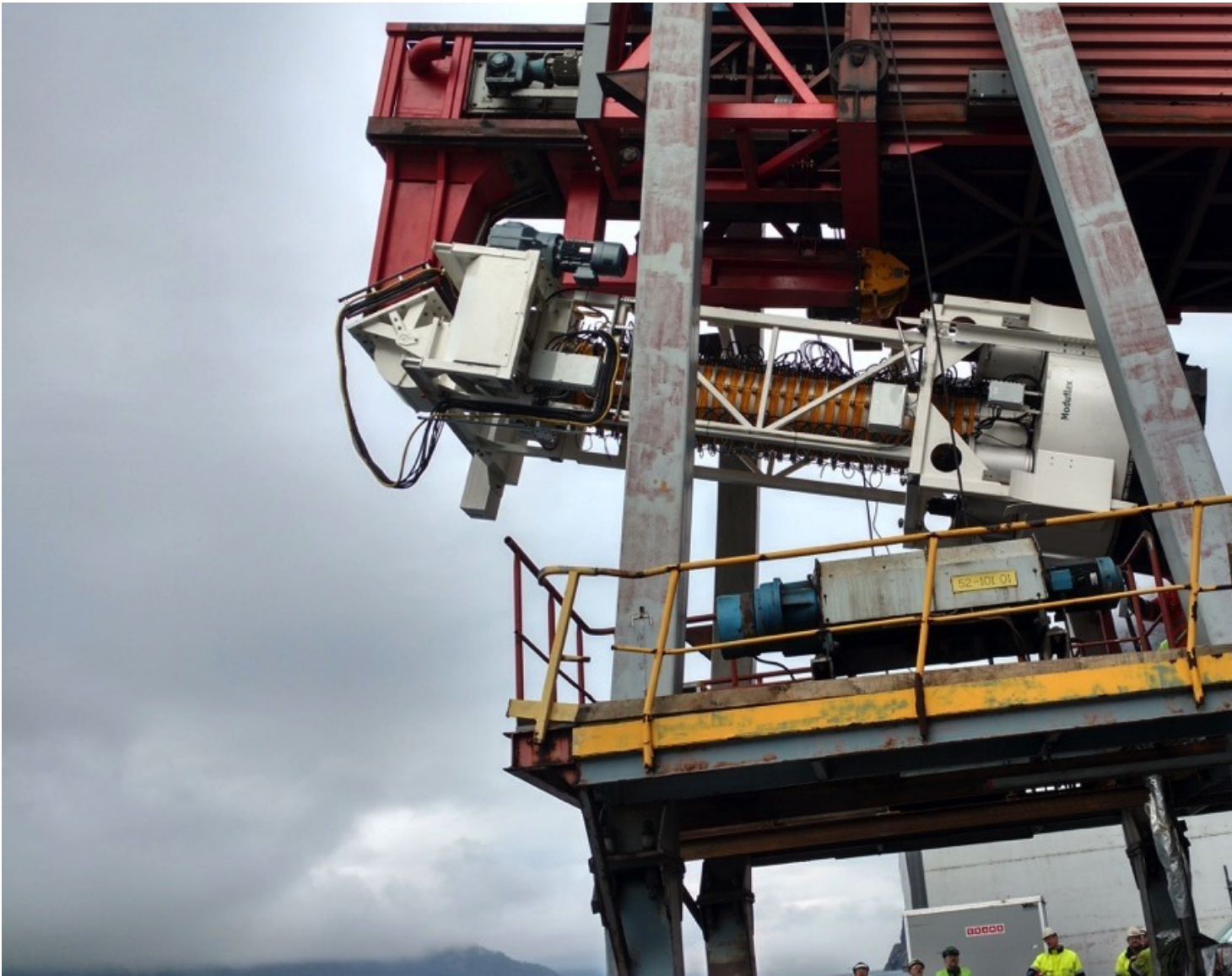
Loading chute with tilting mechanism.
