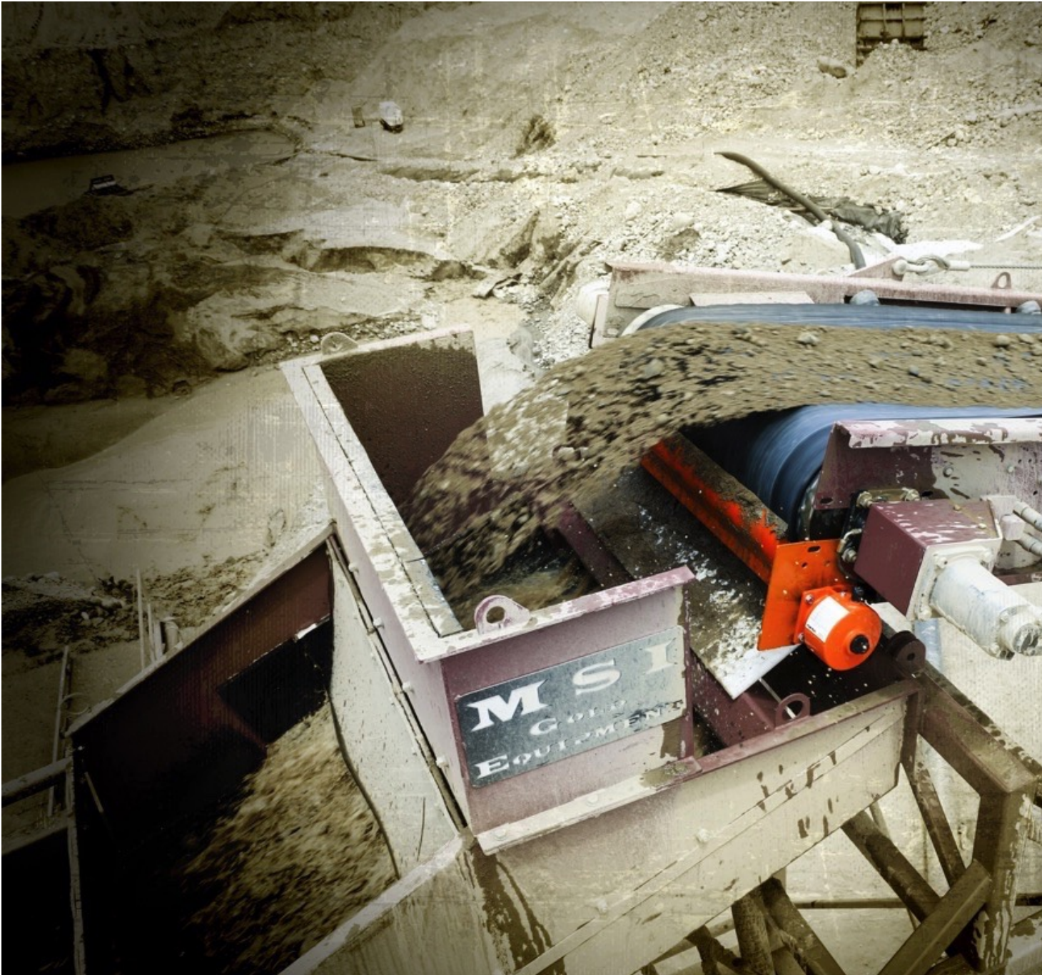
The heavy-duty primary belt cleaner can be replaced safely by one person
